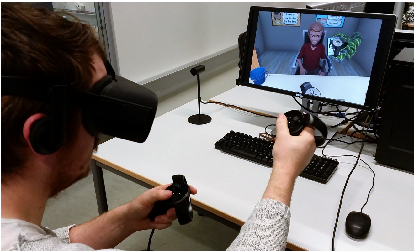
Fig. 2 The system uses the Oculus Rift CV1 head mounted display for full immersion with head tracking and two Oculus Touch VR controllers for picking up and manipulating objects in the virtual environment.
